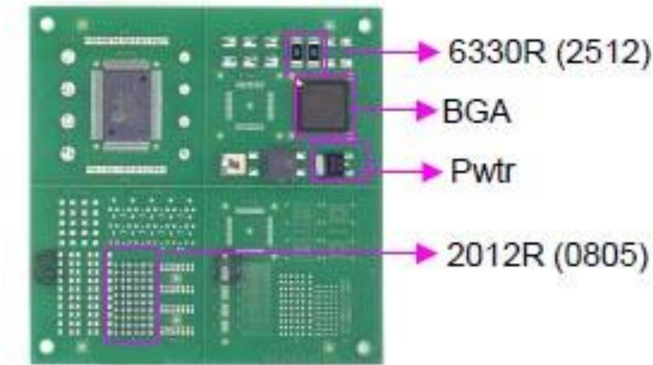
**Figure 8: Company Test Board for Voiding/Reflow Testing**
