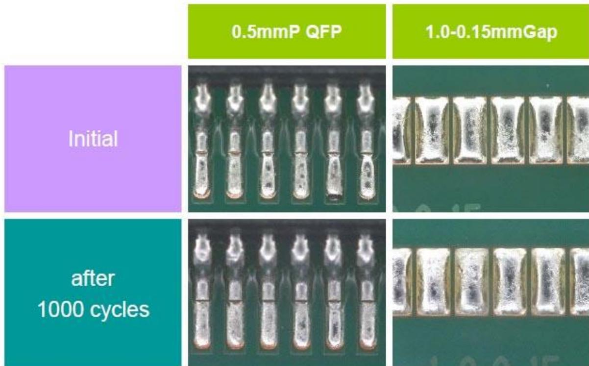
**Figure 9: Cracking test on reflowed crack-free Paste A before and after thermal cycling on soldered 0.5mm pitch QFP component and 1mm wide pads with 0.15mm gaps.**
