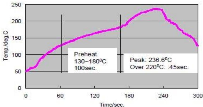
Figure 2: Lead-free reflow profile used
